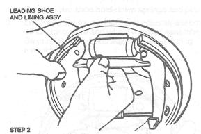
INSTALL ADJUSTER SOCKET TO LEADING SHOE AND LINING ASSY.
