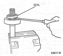
3. Place shaft assembly in arbor press, using Bearing Puller Attachment D84L-1123-A or equivalent, with bearing supported and press out link shaft.
