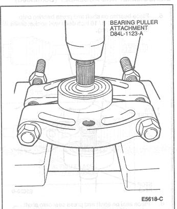
4. Support link shaft in press fixture with step in shaft.
