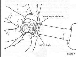
Move stop ring into groove using snap-ring pliers, making sure it is fully seated in groove.
