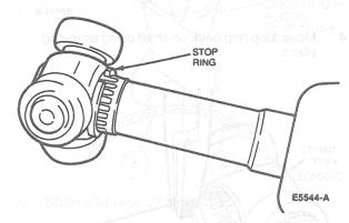
Install trilobe insert over CV joint inner race and position on outer race.
