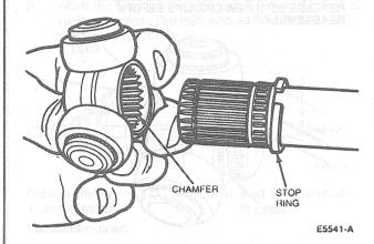
3. Install new circlip.
