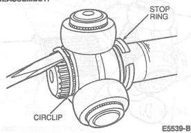
Remove tripod assembly from shaft. Remove boot if necessary.
