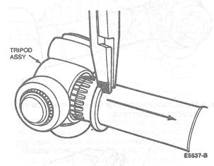
5. Move tripod assembly back on shaft to allow access to circlip.
