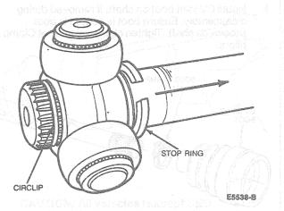
CAUTION: Circlips must not be reused. Replace with new circlips before reassembly
