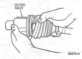
NOTE: Before installing boot clamp, ensure any air pressure which may have built up in boot is relieved. Insert a dulled screwdriver blade between boot and outer bearing race to allow trapped air to escape from boot. The air should be released from the boot only after adjusting to dimension shown in Specifications.
