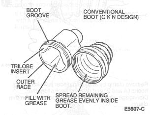
Install outer race on tripod assembly.
