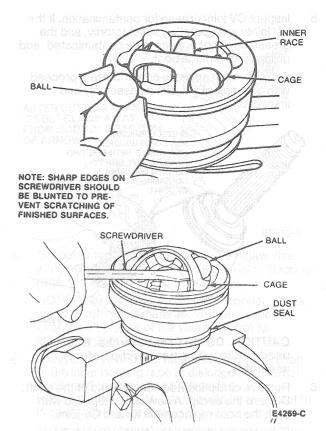
Pivot cage and inner race assembly until it is straight up and down in the outer race. Align cage windows with outer race lands while pivoting the bearing cage.
