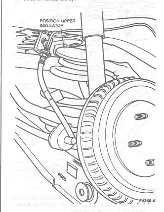
Position spindle in lower suspension arm and install a new bolt, nut, washer and existing cam. Install bolt with the head toward front of vehicle. DO NOT tighten at this time.
