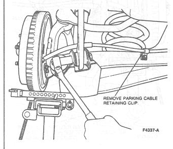
Remove nut, bolt, washer and adjusting cam retaining lower suspension arm to spindle. Discard nut, bolt and washer. 11. Slowly lower suspension arm with floor jack until spring can be removed.
