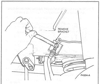
Remove stabilizer bar U-bracket from lower suspension arm.
