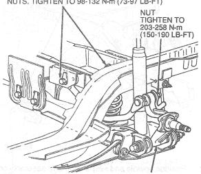
POSITION SPINDLE IN LOWER SUSPENSION ARM. INSTALL NEW BOLT, WASHER, NUT AND EXISTING CAM. TIGHTEN NUT TO 54-71 N-m (40-52 LB-FT) F4333-F
