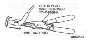
2. When removing wires from distributor cap or coil, grasp boot by hand and remove with twisting and pulling motion. **Do not pull on wire.**
