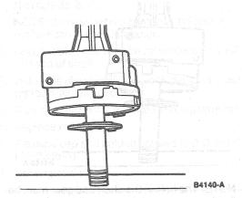
NOTE: The hole in the shaft and gear must be lined up as accurately as possible to ensure ease of roll pin insertion.
