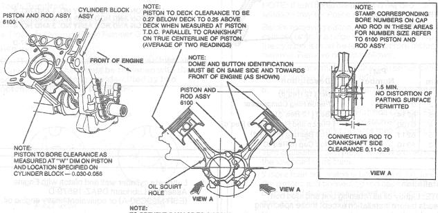
NOTE: TO PREVENT DAMAGE TO PISTONS AFTER ASSEMBLY, POSITION CRANKSHAFT KEYWAY SO ALL PISTONS ARE BELOW DECK
