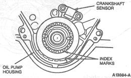
NOTE: The timing belt has three yellow lines. Each line aligns with the index marks shown.
