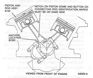
CAUTION: As piston is tapped into bore with a wooden hammer handle, guide connecting rod onto crankshaft journal to avoid damage to bearing surfaces.
