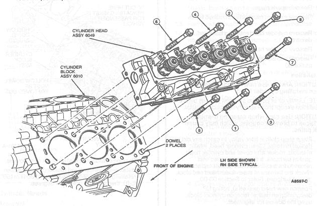
NOTE: When cylinder head retaining bolts have been tightened using the above procedure, it is not necessary to retighten the bolts after extended engine operation. However, the bolts can be checked for tightness if desired.
