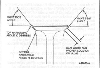
Select proper size pilot and insert it into finished valve guide. Using the 75 degree cutter, make a light cut until a clean line can be seen all the way around bottom of seat angle. Once this is done, use the 30 degree cutter until there is a clean line all the way around top of seat. Then use the 45 degree cutter until seat is clean, free from pits and has an even width all the way around.
