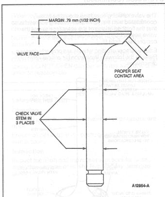
Use Rotunda Motorized Valve Refacer 139-00041 or equivalent, to reface valves. Carefully review instructions supplied with the kit before starting work.
