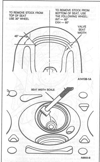
If the valve seat width exceeds the maximum limit, remove enough stock from the top edge and/or bottom edge of seat to reduce the width to specification.
