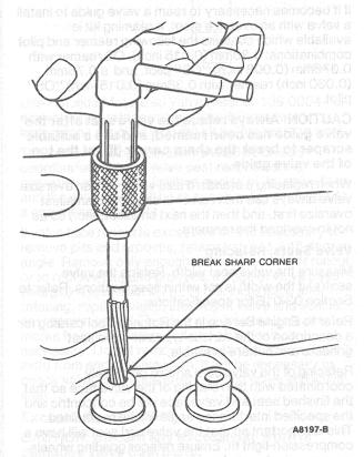
When replacing a standard size valve with an oversize valve always use the reamer in sequence (smallest oversize first, and then next smallest, etc.) so as not to overload the reamers.
