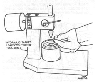
Adjust length of ram so pointer is 1.59mm (1/16 inch) below starting mark when ram contacts tappet plunger, to facilitate timing as pointer passes the Start Timing mark.
