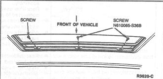
Slide halo and sunshade fully rearward to expose six glass retaining screws (three each side).
