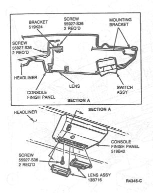
Remove console by sliding up and to rear of vehicle to disengage from mounting bracket.
