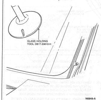
Remove any excess urethane, using care not to smear the urethane on component parts, crash pad and vinyl roof.
