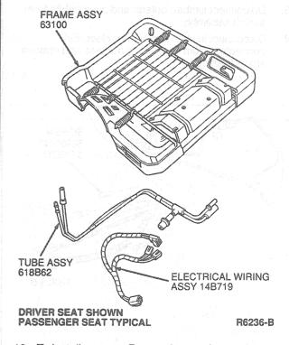
12. To install, reverse Removal procedure.
