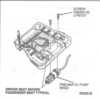
11. Remove electrical harness from cushion frame. Remove tubing assembly from cushion frame.
