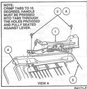
Part Number Description Item 618B47 (Inboard) Track Assy 618B46 (Outboard) Track-to-Seat Retaining Screw (4 Req'd Each Seat) N801078-S58 2A Seat Track Assist Spring 61828 3 Front Seat Track Adjustment Handle 61755 Δ Spring Assy-Front Seat Cushion 5 63100 Tighten to 17-23 N·m (13-17 Lb-Ft) Α
