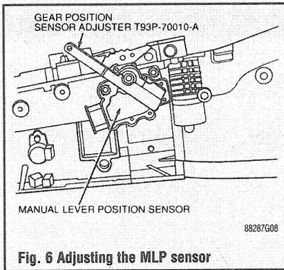
Fig. 6 Adjusting the MLP sensor
