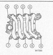
Fig. 49 Intake manifold bolt torque sequence—4.6L engine
