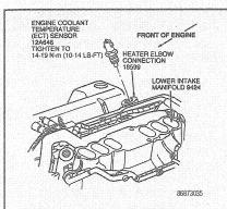
Fig. 46 Location of engine coolant temperature sensor—3.8L engine
