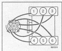
Fig. 34 3.8L Engine Firing Order 1-4-2-5-3-6
