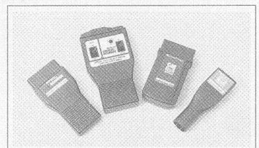
**Trouble code tools** allow the home mechanic to extract the "fault code" number from an on-board computer that has sensed a problem (usually indicated by a Check Engine light). Armed with this code, the home mechanic can focus attention on a suspect system or component
