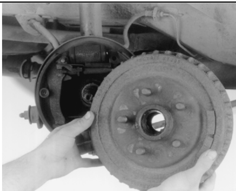
Remove the rear hub and drum assembly from the spindle
