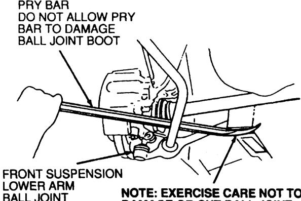
NOTE: EXERCISE CARE NOT TO DAMAGE OR CUT BALL JOINT BOOT. PRY BAR MUST NOT CONTACT LOWER ARM.
