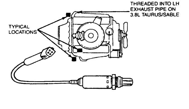
THREADED INTO CENTER REAR OF EXHAUST MANIFOLD ON 2.3L HSC, 2.5L THREADED INTO Y-PIPE JUNCTURE OF CATALYST INLET ON 3.0L EFI/
