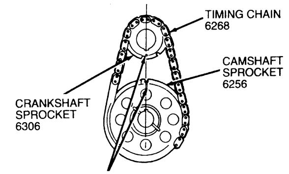
POSITIONING OF TIMING MARKS AND KEYWAYS IN CAMSHAFT AND CRANKSHAFT SPROCKETS MUST BE IN LINE AS SHOWN WITH NO. 1 PISTON AT TOP DEAD CENTER FIRING
