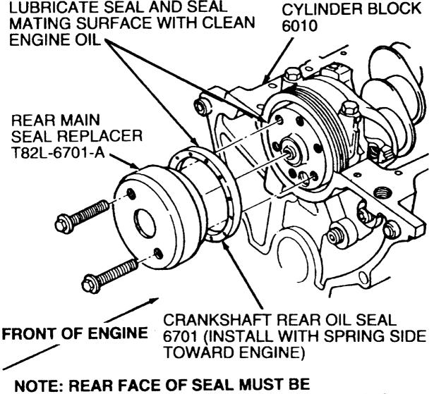
NOTE: REAR FACE OF SEAL MUST BE WITHIN 0.508 mm (0.020 mm INCH) OF THE REAR FACE OF THE BLOCK
