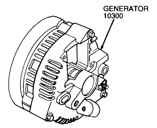
VOLTAGE REGULATOR 10316 AND GENERATOR BRUSH AND TERMINAL HOLDER 10320
