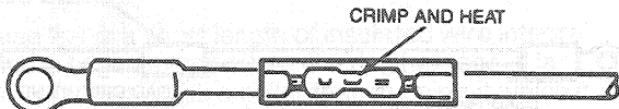
TYPICAL REPAIR USING THE EYELET TERMINAL FUSE LINK OF THE SPECIFIED GAUGE FOR ATTACHMENT TO A CIRCUIT WIRE END J2323-C
