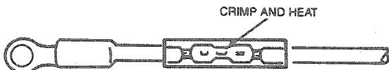
TYPICAL REPAIR USING THE EYELET TERMINAL FUSE LINK OF THE SPECIFIED GAUGE FOR ATTACHMENT TO A CIRCUIT WIRE END J2323-C
