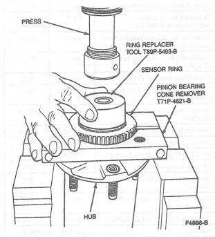
2. Press anti-lock sensor ring off of hub assembly.
