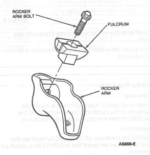
CAUTION: Do not attempt to true-up this surface by grinding. On pedestal mounted rocker arms, check the rocker arm pad, side rails and fulcrum seat for excessive wear, cracks, nicks or burrs. Check the rocker arm bolt for stripped or broken threads.
