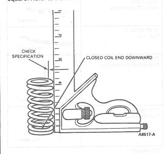
Refer to Specifications in Section 03-01B for out-of-square limits. Follow the same procedure to check new valve springs before installation.
