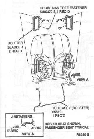
12. Remove two screws from each bolster guide and brackets on seat back frame. Disconnect the bottom of two springs from the seat back frame at the left bolster opening and two springs from the seat back frame at the right bolster opening.
