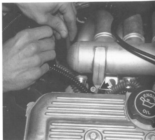
Fig. 2-15. Checking injector triggering by control module using a Light Emitting Diode (LED) test light (arrow).
