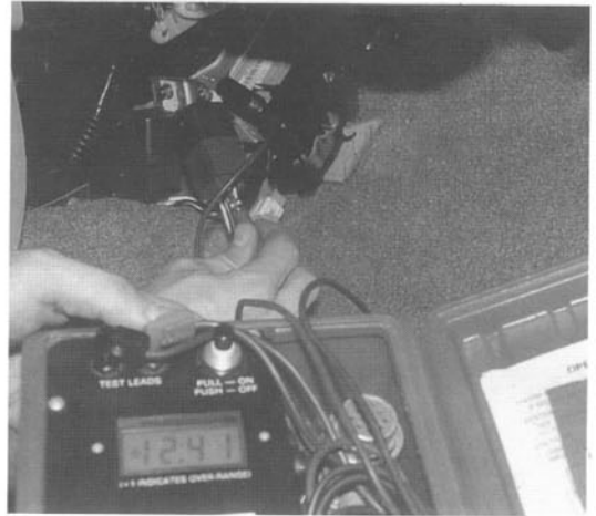
Fig. 2-6. Check voltage at fuel-pump relay. On the '91 1.9L Escort, it is under the center console.
