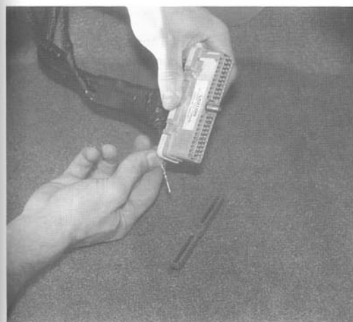
Fig. 3-2. Control module harness connector being back-probed to test pins (or use BreakOut Box).
