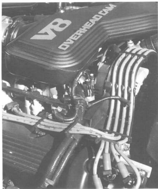
Fig. 2-14. Ford identifies cylinder numbers differently from other manufacturers. It pays to check the diagrams or the cylinder number identifiers on the plug wires of late-model engines.
