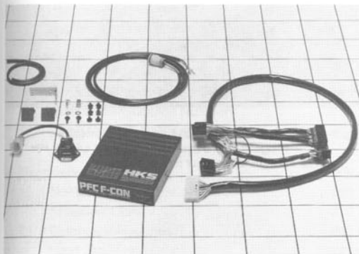
Fig. 8-2. HKS power chip module monitors Ford control module and modifies injector pulse times. Not certified for street use.
