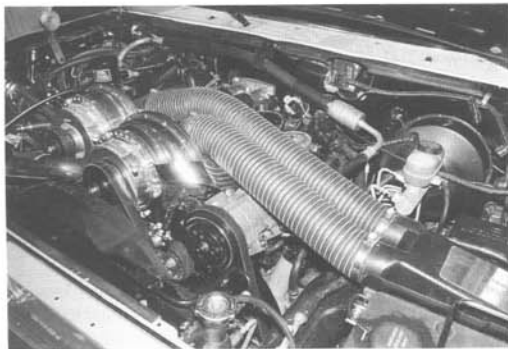
Fig. 6-11. Paxton twin-supercharger kit for large-displacement engines provides over twice the volume of air over single 5.0L unit. Kit pending CARB exemption.
