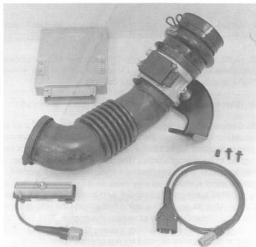
Fig. 4-1. Mass Air Flow (MAF) kit converts Manifold-Absolute Pressure (MAP) system from indirect sensing of air-flow to direct sensing for performance mods. Includes new EEC-IV control unit.
