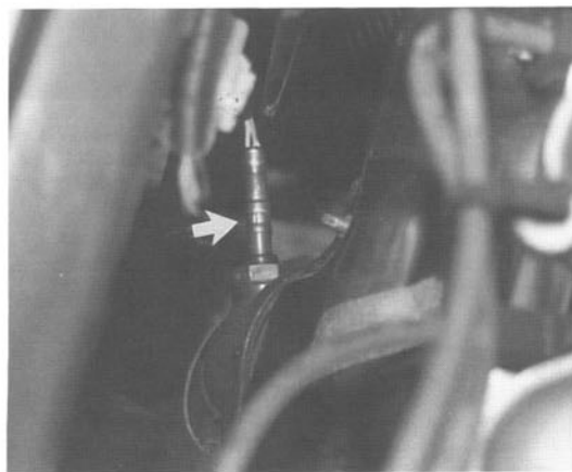
Fig. 6-1. Oxygen sensor generates its own voltage when air-fuel ratio is rich, but only when sensor is hot. Oxygen sensor threads into exhaust manifold where it samples oxygen content in hot exhaust gasses.
