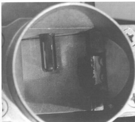
Fig. 3-14. Air Charge Temperature (ACT) sensor in VAF signals temperature of incoming air. Together with pressure signals from BP, these measurements can be combined in control module to calculate air mass.
