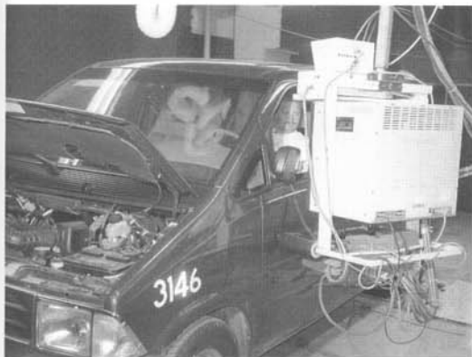
Fig. 2-3. Every car and light truck engine is certified to meet EPA emissions standards, and from those measurements, standards for fuel economy. Drivers follow exact driving pattern. Dynamometer rolls load engine according to inertia weight and resistance to movement, including friction, tire rolling resistance, and aerodynamic drag.
