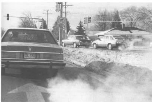
Fig. 2-2. Tailpipe steam is visible when natural water vapor, H_2O , condenses in cold air. Pollution is normally not visible, and what's visible is not necessarily pollution.
