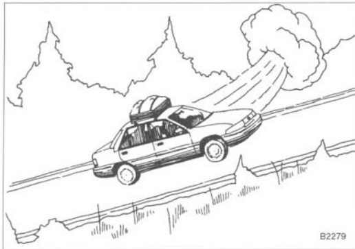
Fig. 2-10. Load changes as a result of hill, head wind, trailer, truck load, also under-inflated tires, open windows, dragging brakes, luggage/ski racks, etc.
