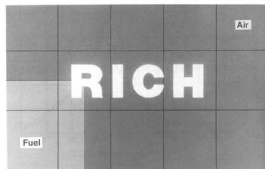
Fig. 2-3. A rich mixture burns almost all the oxygen, so exhaust gas is low in oxygen content. Exhaust gas has much unburned fuel.
