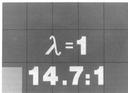
Fig. 2-5. For a warm engine, running on gasoline at part throttle, the ideal or "stoichiometric" air-fuel ratio—when there is just enough air to burn all the fuel—is 14.7:1.
