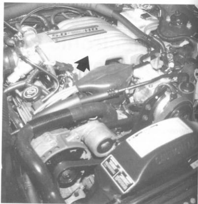
Fig. 1-2. MFI (Multiport Fuel Injection) is often hidden by manifold runners (arrow).
