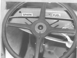
Fig. 4-2. Ford Model A driver controlled spark timing and fuel directly. EEC systems control timing and fuel to satisfy many requirements, many times per second.
