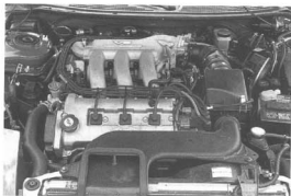
Fig. 3-2. MEC-II controls 2.5L V-6 in 1993 Probes. Also 2.0L 4-cylinder with automatic transmission (4EAT).
