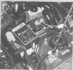
Fig. 1-3. Scan tool is plugged into diagnostic connector to read trouble codes. Analog voltmeter can also be used. Reading trouble codes is essential to troubleshooting electronic engine control.
