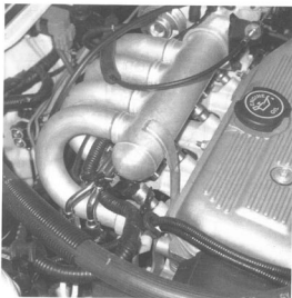
Fig. 3-5. Long intake runners, called ram manifolds, are widely used in Ford fuel injection.
