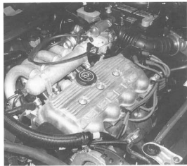
Fig. 2-1. Electronic control of fuel injection and ignition helps clean up the tangle of underhood hoses that are necessary when vacuum circuits are used.
