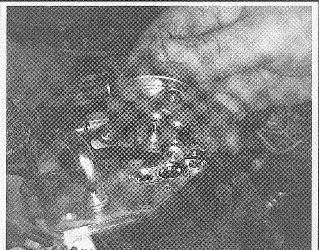
Fig. 45 . . . lift the regulator off of the rail
