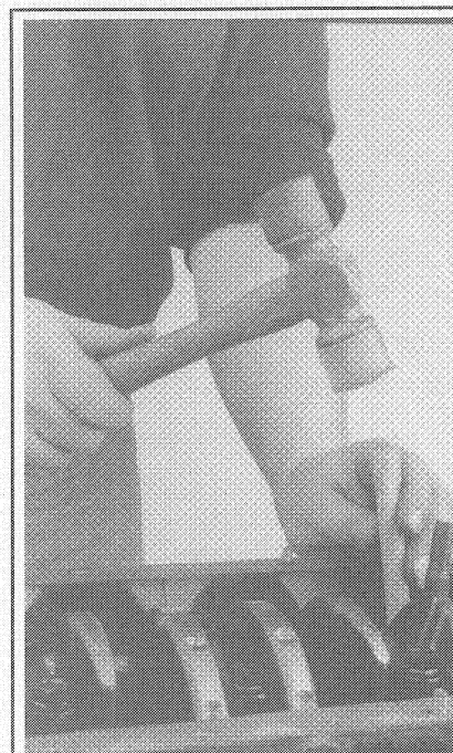
Fig. 208 Carefully tap the piston out of the bore using a wooden dowel
